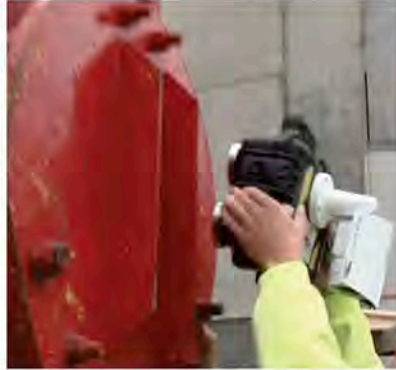
HoistCam Installed on Crane's Hook Block (HC110)
